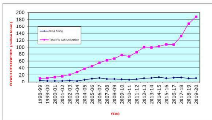
Figure 1 : Shows the progressive utilization of fly ash in mine back filling/ stowing during the period 1998-99 to 2019-20 [Source : CEA(2020)]
