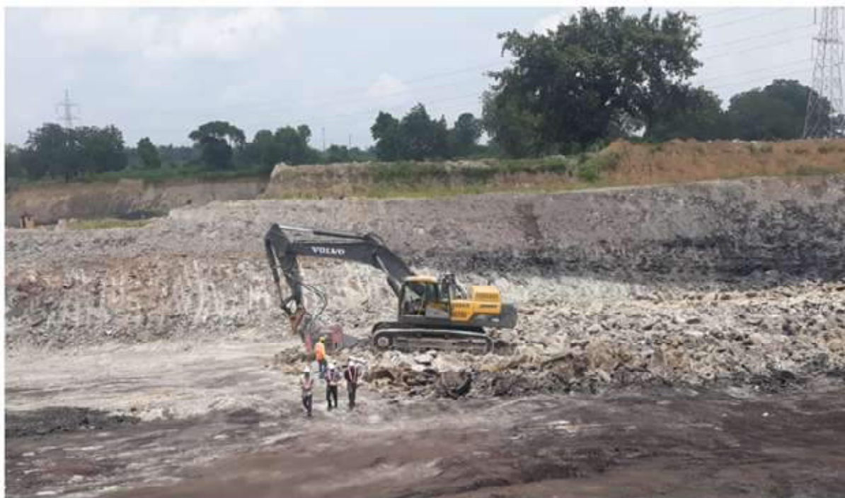
Fig. 1 : Showing deployment of X-centric/vertical ripper attachment mounted on Hydraulic Excavator in operation at sandstone OB bench
