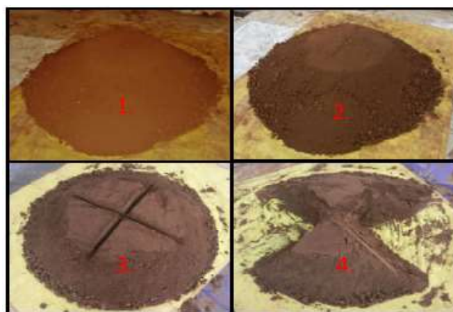
Fig 1: Coning and quartering of waste dump sample
