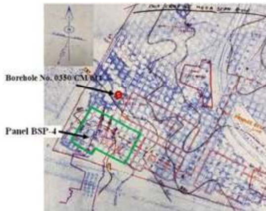
Fig. 1: Part plan of developed Bogra seam (R-VI) showing the location of proposed depillaring panel BSP-4.
