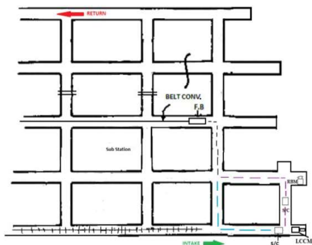
Fig. 5: Layout for 5-Heading Development District with LCCM
