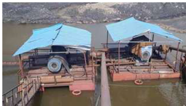
Fig.6: Pontoon Pumping of dewatering in mines
