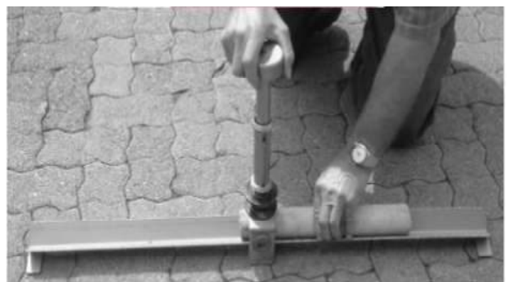
Figure 4 : The Impact Splitting Test setup
