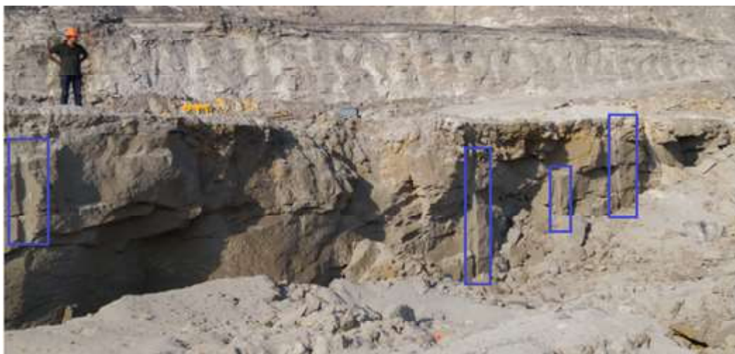
Fig. 9: Half cast impressions achieved in dragline bench
