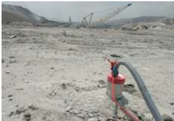
Fig. 5: Field placement of near-field sensor
