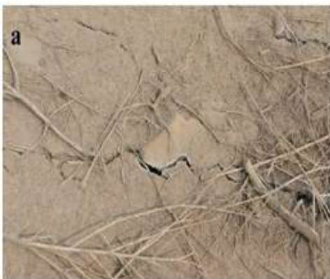
Fig. 7A: Crack due to underground coal mines fire March 2021
