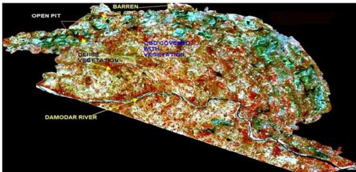
Fig. 2: Landsat 8 OLI false colour composite image of Jharia Coalfield (R: NIR, G: Red, B: Green) date of acquisition (2 Feb 2015)
