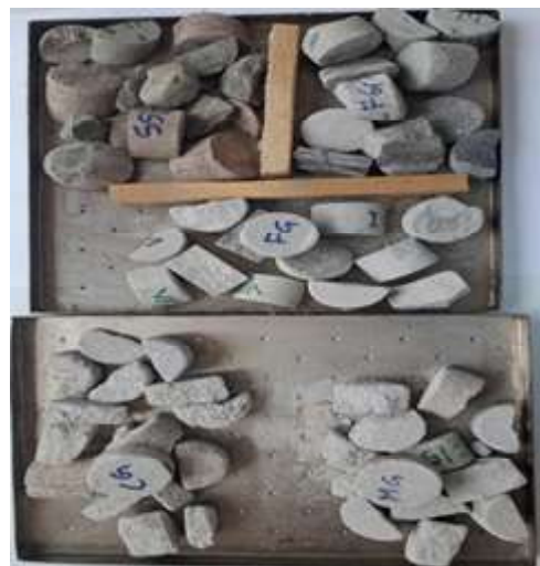
Figure 2 : Rock Samples for Slake Durability Index Test
