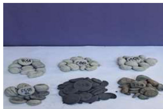
Figure 5 : Coal Measure Rock Samples After Slake Durability Test
