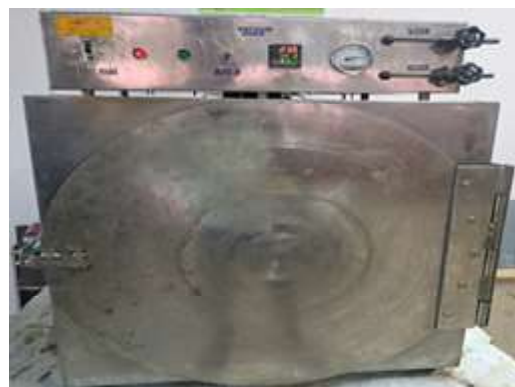
Figure 3 : Vacuum Oven for Drying the Rock Samples
