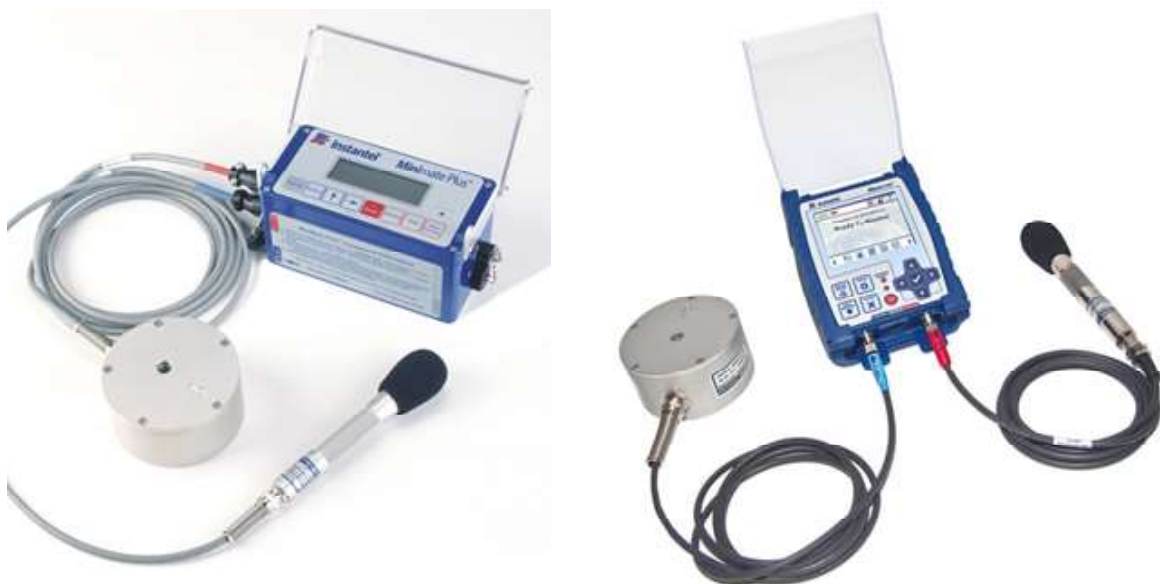
Fig. 4: View of MinMate Plus and Micromate Equipment along with external geophone and microphone sensors
